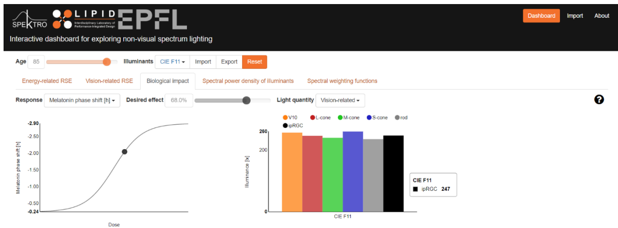
Figure 17. Dose response curve for an 85 years old individual, with a CIE F11 light source and a 68% desired effect on circadian resetting (EPFL-LIPID, 2015).
