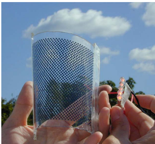
Sphelar spherical solar cells, © Kyosemi
