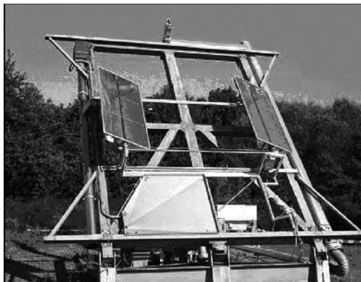
Figure 4. Testing of two PTC 1000 modular parabolic trough collectors at DLR in Germany. In these tests, the collectors are installed on a tilted testing platform to eliminate the effect of end-losses.
