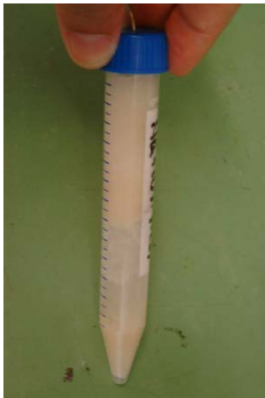
Figure 8: Segregation of a salt hydrate
