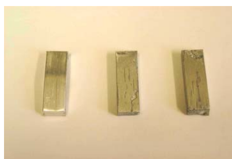
Figure 7: Aluminium treated with a salt hydrate. From left to right: before treatment, after treatment, and after treatment in contact with graphite
