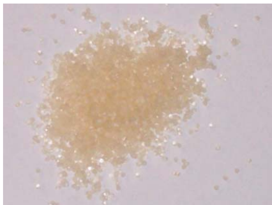
Figure 10: Microencapsulated PCM by copolymerization
