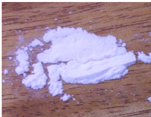
Figure 11: Microencapsulated PCM commercialized by BASF
