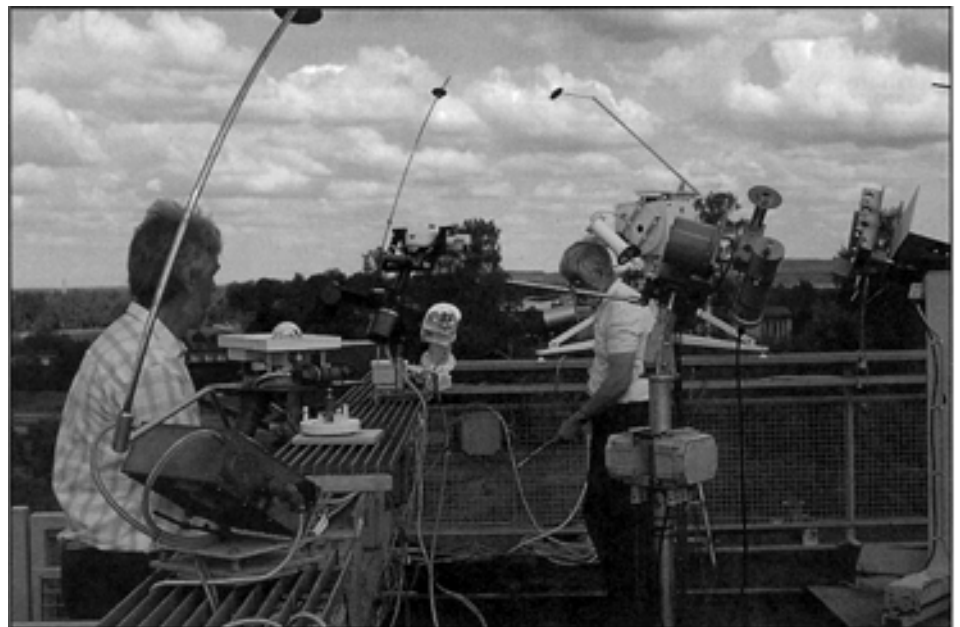
Outdoor comparison of global solar radiation reference radiometers (GRRR) at Norrköping, Sweden. The GRRR, developed by Task 9 experts, has proved to be the most accurate system for measuring global solar radiation.
