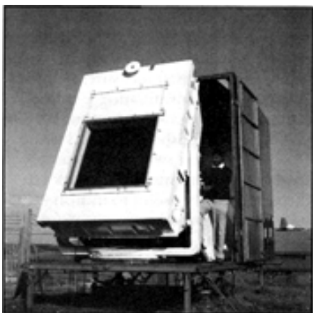
Solar Calorimeter at the University of New South Wales used to test a wide range of window types.
