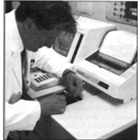
Spectrophotometer tests will be performed in Task 18 to measure optical properties of advanced glazings.
