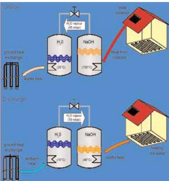
A schematic of NaOH storage.
