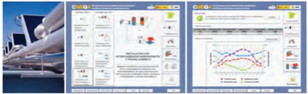
▲ Figure 3. CHEQ4, a software package to promote solar thermal systems compliance with the Spanish Building Technical Code (Source: http://www.codigotecnico.org/index.php/cheq4 ).
