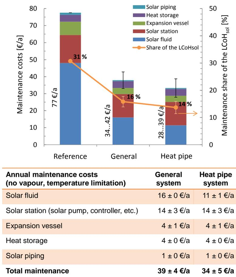
Figure 2: Annual maintenance costs of both optimized systems (general and heat pipe) compared to the reference system as well as their share of the Levelized Cost of Heat ( $LCoH_{sol,fin}$ )
