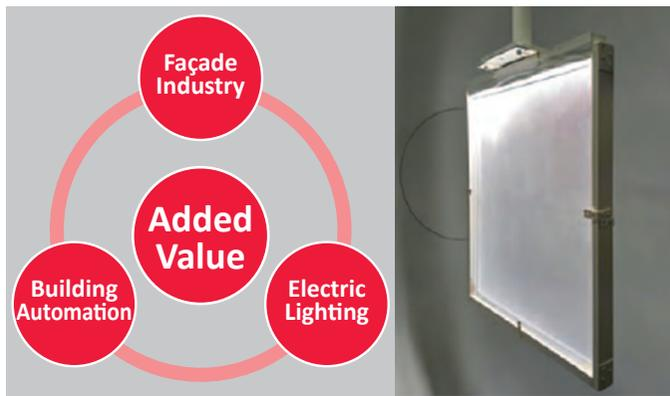
The task will work on integrating different building sectors involved (left). Example of a new integrated façade component, transmitting daylight while at the same time emitting electric light (right).
