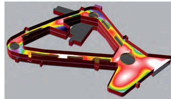
Example of integrated daylighting and electric lighting design.
