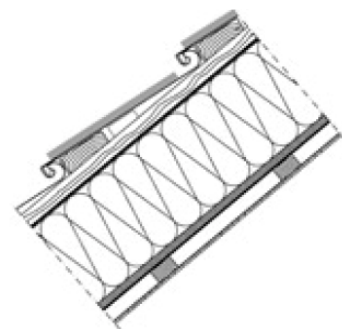
Design structure of QUICKSTEP RHEINZINK® Stepped Roof
