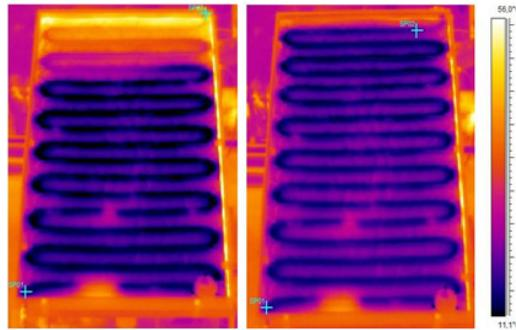
Fig. 5. Thermographs of the absorber plate
