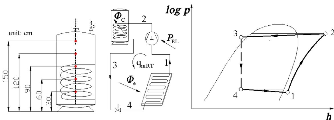
Fig. 2. Positions of thermocouples in the water tank and heat pump cycle in the  $\log p, h$  diagram
