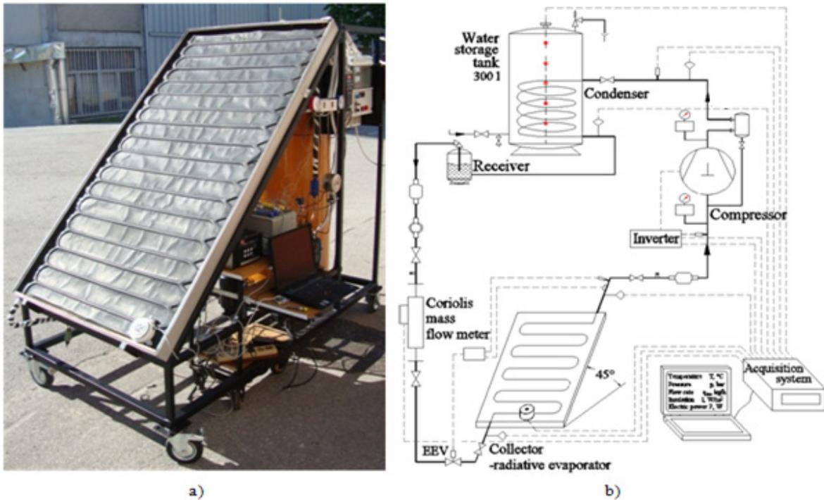
Fig. 1. Mobile DX-SAHP: a) unit in operation; b) schematic diagram of the developed unit
