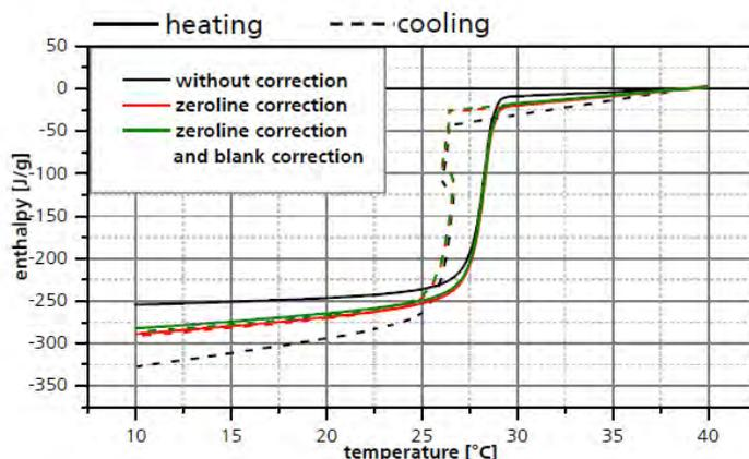
Further improvements in the "Measurement procedure Phase Change Materials Task 42/29" were achieved by introducing a zero-line and blank correction in the evaluation of the measured data.
