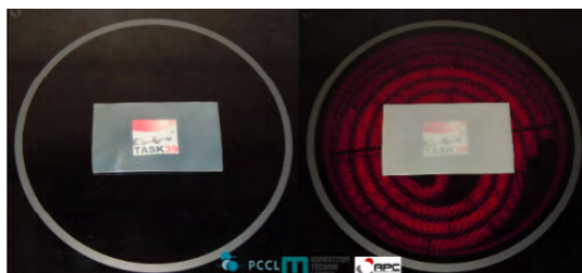
Figure 1c. Thermotropic layer in transparent and opaque state (PCCL, Leoben, Austria).
