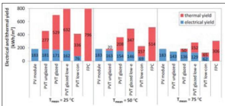
◀ **Figure 8. PVT collectors maximize the solar energy collected at all temperatures. The temperature influence in thermal and electrical gains per square meter of collector aperture area calculated using the software “ScenoCalc” for the city of Würzburg, Germany (Central Europe).** (Source: IEA SHC Task 60 report, Status Quo of PVT Characterization)
