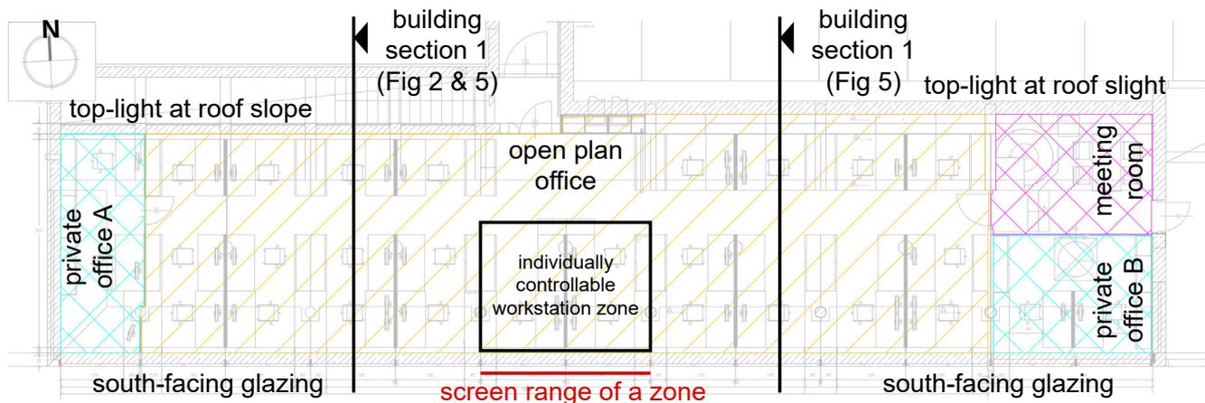
Figure 2. Floor plan of the Bartenbach R&D building.
