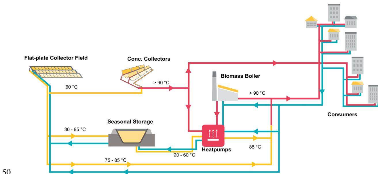
Fig. 1: Possible concept for future solar district heating systems efficiently providing the heat at the desired temperature
