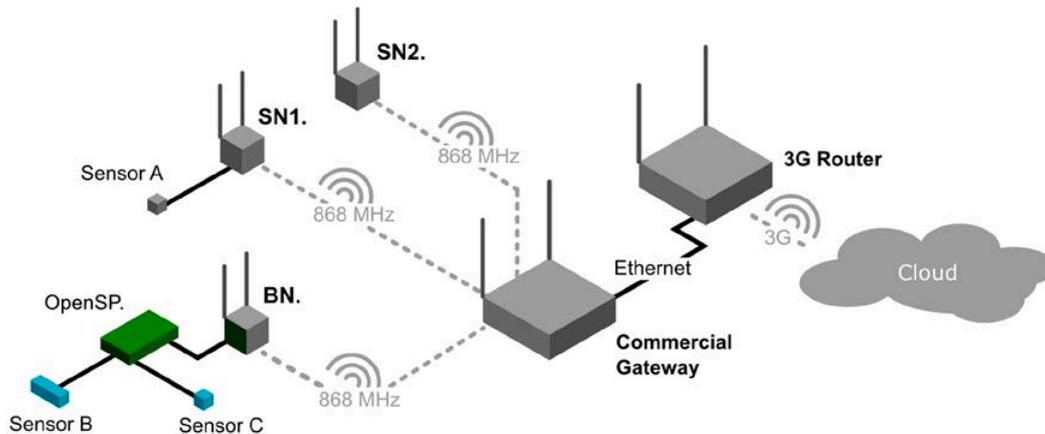
Figure 5. The flexibility of the 'hybrid' WSN system for the monitoring of heritage buildings. SN1 = Commercial sensor node with external sensor; SN2 = Commercial sensor node with internal sensor; BN = Commercial bridge node; OpenSP = Open source signal-processing unit.
