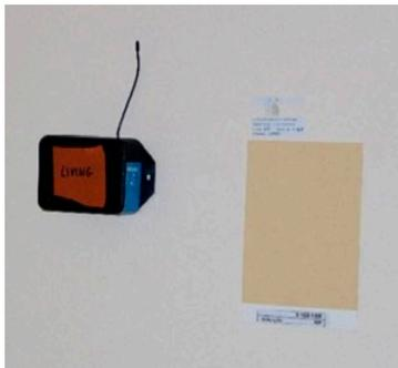
Figure 6. A temperature and humidity sensor node (commercial system) mounted on an interior wall in building B.
