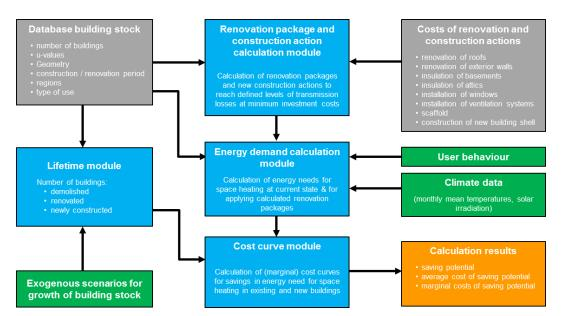
Figure 1: Structure of the calculation process to derive cost curves with the Invert/EE-Lab model
