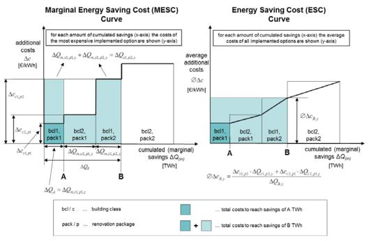
Figure 2: Exemplary Marginal Energy Saving Cost (MESC) curve and Energy Saving Cost (ESC) Curve for two building classes and two renovation packages per class
