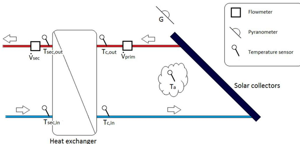
Fig. 2. Schematic drawing showing the measurement points.  $T_{c,out} = T_{prim,in}$  and  $T_{c,in} = T_{prim,out}$ .
