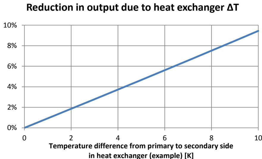
Figure 1. Example of the influence of the heat exchanger on the performance of the solar system. The higher the temperature difference across the heat exchanger ( $\Delta T$ ) the higher the temperature in the collector loop - and the lower the collector performance. The influence of the heat exchanger depends on the heat loss coefficient of the solar collector: The higher the collector heat loss coefficient - the larger the influence of the heat exchanger. (Source: PlanEnergi)
