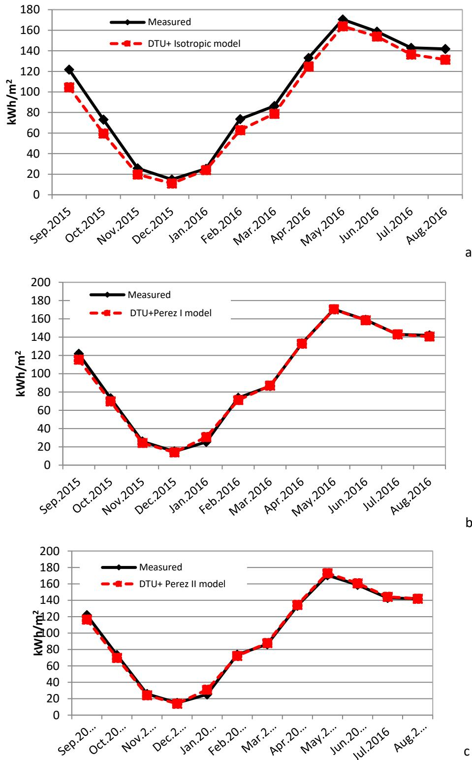
Fig.9. Measured monthly tilted total radiation and calculated tilted total radiation based on calculated
