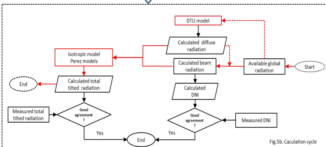
Fig.5.Schematic illustration of the methodology (Fig.5a.Validation cycle, Fig.5b.Caculation cycle). [29]
