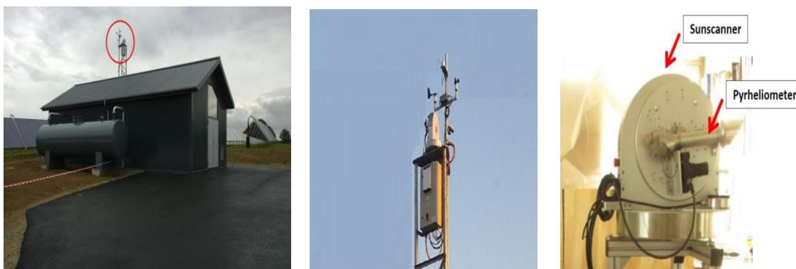
Fig.4. Used weather station and pyrheliometer of the Tårs solar heating plant [29]
