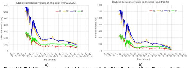
Figure 4.18: Global illuminance values (a) and daylight contribution (b) on the desks of the multi-occupant's office acquire on 10/03/2020.
