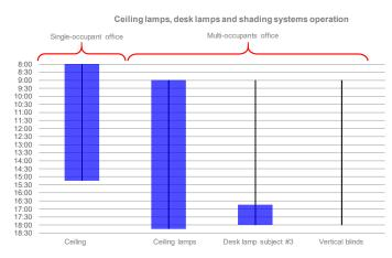
Figure 4.14: Operation of ceiling lamps, desk lamps and shading systems for both offices.
