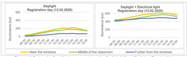
Figure 4.49 Registration Day, illuminance on task position Daylight (left) and Daylight + Electrical light
