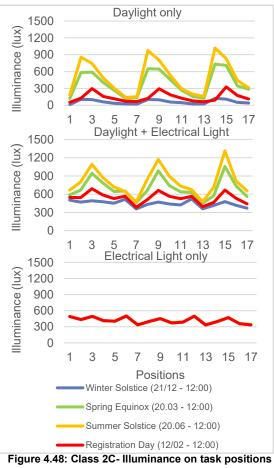
for the combination of daylight and electrical light, the illuminance uniformity reaches 0,59 to 0,80.
