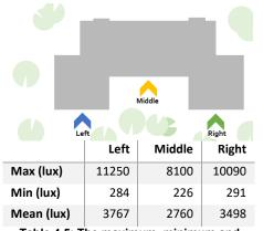
Table 4.5: The maximum, minimum and mean amount of illuminance on facade for each measurement location.
