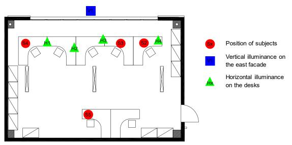
Figure 4.12: Detailed view of the multi-occupant office with an indication about the indoor illuminance values measurement points as well as the position of the employees.
