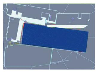
Distribution of PV on the roof of Building 23 (788 kWp) and parking (740 kWP). Source: s2e Technologies Inc.
