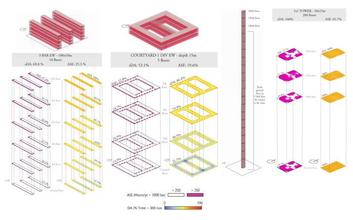
Example of one type of simulation using DIVA (Solemma): Spatial Daylight Autonomy
