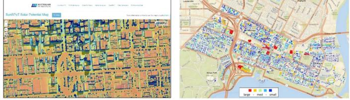
APVI Solar Potential Tool (SunSPoT) Map representation (left) and Perth CBD rooftops with the largest PV potential (right)
