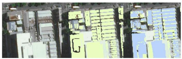
Example of good agreement between the two input data sources for large buildings. Aerial image (Left), AAM 3D buildings with Insolation limit method (centre); LiDAR with Insolation limit method (Right)
