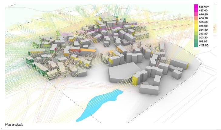
The daylight access was in this project studied as the amount of solar hours on facades at equinox (~March 20 & September 23). In other projects, the architects have used the Vertical Daylight Factor.
