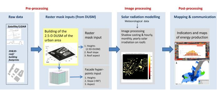
Workflow of the whole process of solar modelling on roofs and facades. Source: https://doi.org/10.3390/app10155361
