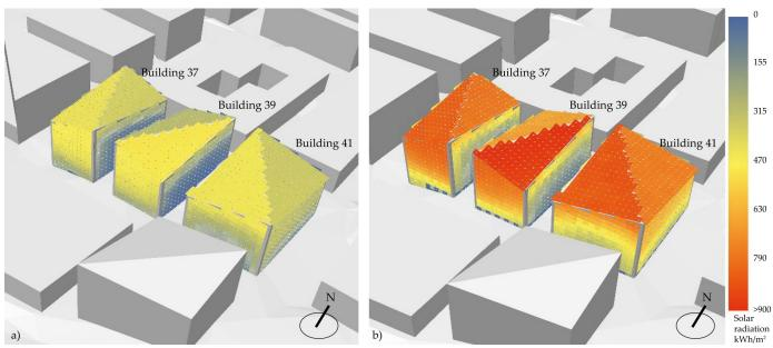
Annual grid-based analysis of direct solar irradiation (a) and global irradiation (b) in the critical area for Feasibility Study I
