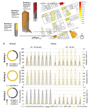
Heat map of the annual ST-PV window potential of area number 5 and seasonal PV performance of selected buildings. a. ST-PV window potential to building footprint area ratio (kWh m2 a-1) and the selection of high-performing buildings b. Doughnut chart of the annual PV production and hourly PV performance of a typical winter and summer week.
