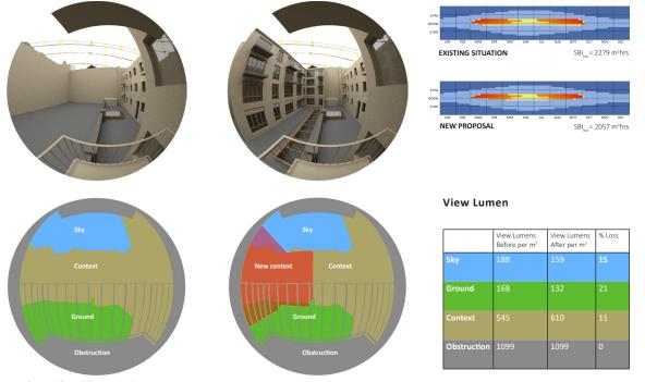
Aperture Based Daylight analysis
