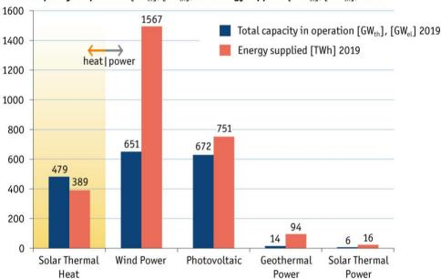
Global capacity in operation [GW<sub>el</sub>], [GW<sub>th</sub>], and energy supplied [TWh<sub>el</sub>], [Twh<sub>th</sub>], 2019
