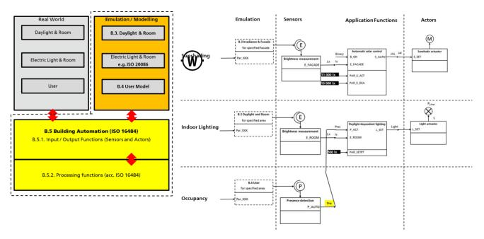
Emulation concept and structure of the comprehensive hourly method and an example of the model structure for a fully automated single office.
