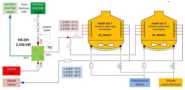
Figure 8: Solar heat and biomass district heat integration into the mash tuns of Goess brewery (Mauthner et al. 2014)
