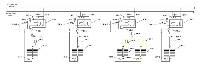
Figure 10: Four separate solar thermal systems installed for each heat demanding process. (from left to right) System 4, System 3, System 2, System 1. (Source: Aspiration Energy)
