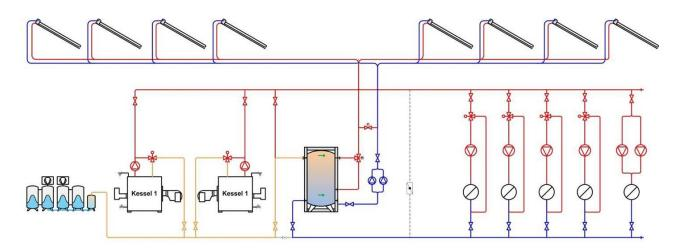
Figure 14: Integration of the evacuated tube collector field into the heating network parallel to the existing boilers (Source: Ritter XL Solar)
