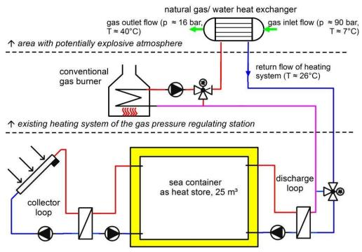
↑solar thermal system in return flow of the existing heating system
