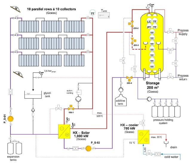
Figure 7: System concept of the SPH installation at Goess Brewery (Source: AEE INTEC)
