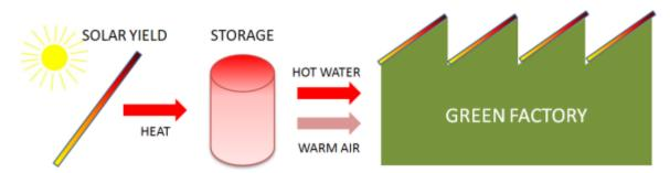
Fig. 11: Principle of solar process heating
