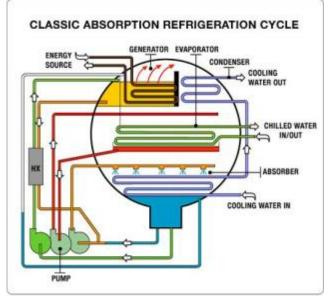
Fig. 4: Schematic of an absorption chiller [2]
