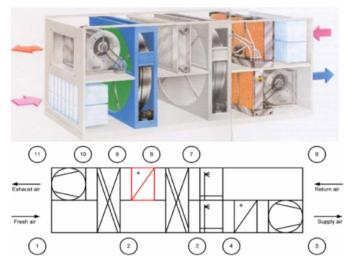
*Fig. 8: Schematic of an Desiccant cooling system* <u>Cooling cycle</u>
