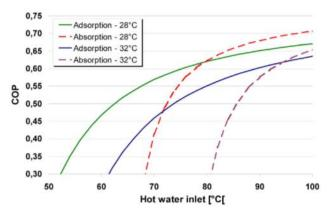
*Fig. 7: COP of adsorption and absorption chiller as a function of heating water temperature (chilled water 9°C,cooling water 28 and 32 °C);* [*Error! Bookmark not defined.*]
