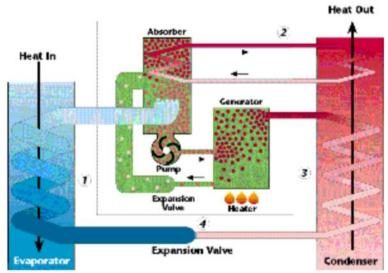
Fig. 16: Absorption heat pump
