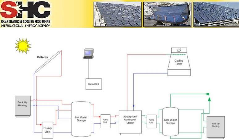
*Fig. 3: Solar cooling schematic*
