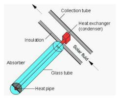
Figure 9: Evacuated Tube Collector<sup>17</sup>
