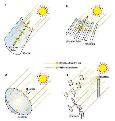
Figure 8: Concentrating Collector Types<sup>16</sup>
