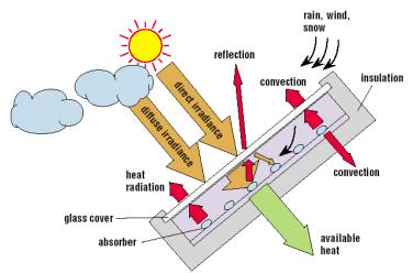
Figure 7: Flat Plate Collector<sup>15</sup>
