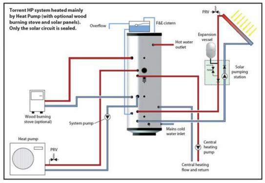
Figure 13: Solar Combination Systems<sup>21</sup>
