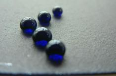
Colored TISS coating on PPS absorber (left) and colored water droplets on TISS paint surface (right).
