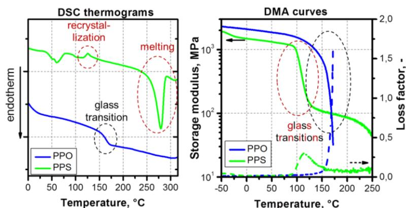
crystallizing semi-crystalline plastics such as PPS is an exothermic recrystallization peak between glass transition and melting range. For PPS recrystallization takes place around 130°C. To avoid physical changes in the use phase and to improve the mechanical properties PPS components are commonly tempered at elevated temperatures around 140°C.
