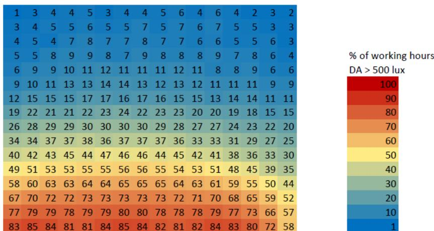
Figure 29: Dynamic Daylight Autonomy for the refurbished case-study (IES-VE)
