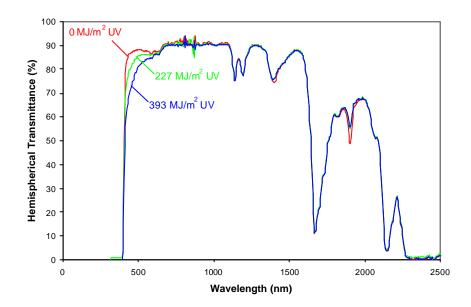
Figure 2 Change in hemispherical transmittance as a function of cumulative UV dose for UVstabalized polycarbonate
