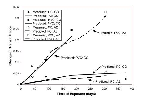
Figure 3 Measured vs. predicted change in hemispherical transmittance between 400-500 nm for two polymeric materials at two outdoor exposure sites.
