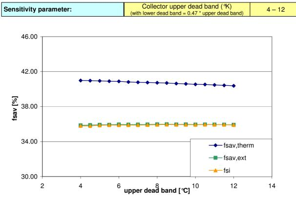
Figure 10: Variation of fractional energy savings with collector upper dead band with lower dead band = 0.47 upper dead band
