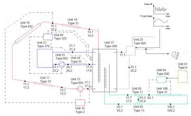
Figure 2: Modelling of the MaxLean system in TRNSYS
