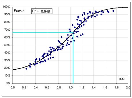
Figure 15: Variation of fractional energy savings with the fractional solar consumption (FSC`) with fixed storage size of 800 litres and different collector areas for 4 climates (Zurich, Barcelona, Madrid, Stockholm) and 4 buildings
