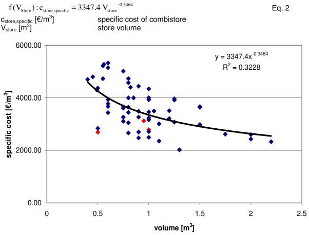
Figure 11: Specific cost of solar combisystems
