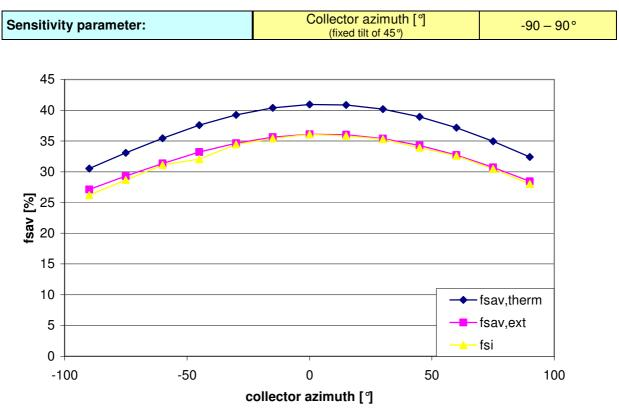
Figure 7: Variation of fractional energy savings with collector azimuth with fixed tilt of 45°
