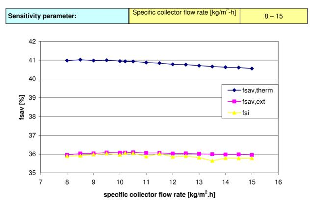
Figure 9: Variation of fractional energy savings with specific collector flow rate
