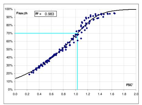
Figure 14: Variation of fractional energy savings with the fractional solar consumption (FSC`) with specific storage volume of 70 I/m<sup>2</sup> for 4 climates (Zurich, Barcelona, Madrid, Stockholm) and 4 buildings
