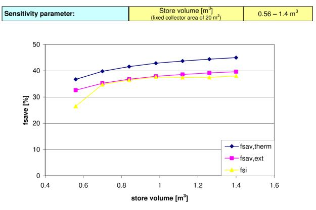
Figure 6: Variation of fractional energy savings with store volume with fixed collector area of 20  $\ensuremath{m^2}$
