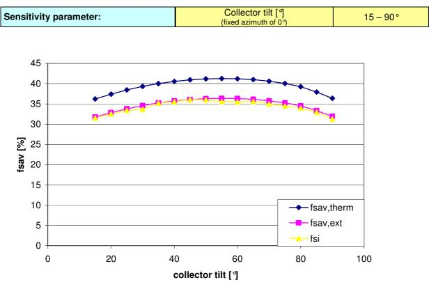
Figure 8: Variation of fractional energy savings with collector tilt with fixed azimuth of 0°
