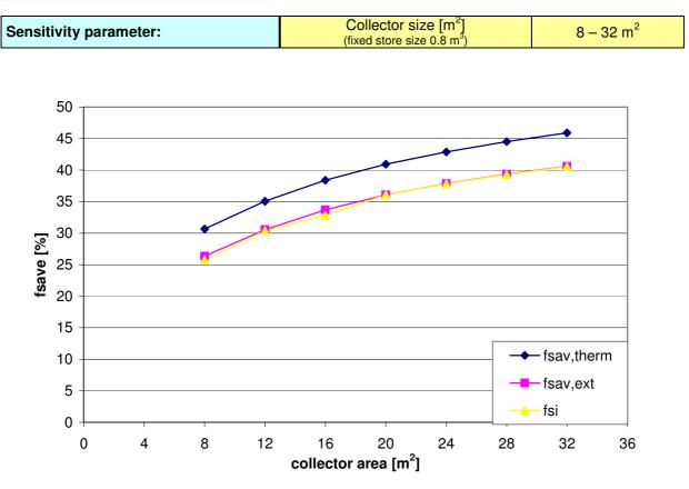
Figure 4: Variation of fractional energy savings with collector size with fixed store volume of  $0.8 \text{ m}^3$ .
