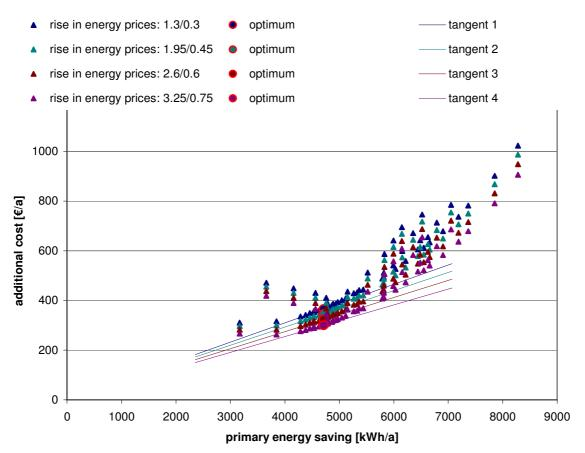
Figure 13: Dimensioning of the MaxLean system with different rises in energy prices
