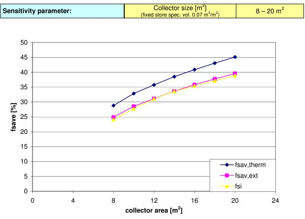
Figure 5: Variation of fractional energy savings with collector size with specific store volume of 0.07  $m^3\!/m^2$
