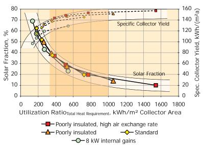
signify low degrees of solar fraction and vice versa. The specific yield shows the well-known behavior running contrary to the solar fraction.
