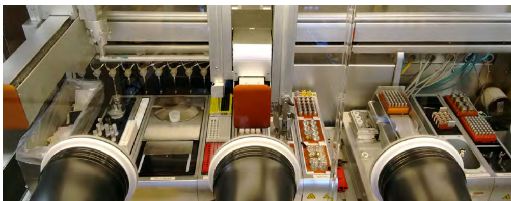
Figure 6.2 HERMAN. Robotic deck of HERMAN, the High-through Experimentation Robot for Multiplexed Automation of Nanochemistry. HERMAN, the successor of WANDA, is used to synthesize colloidal inorganic nanomaterials and nanocomposites at the Molecular Foundry (Lawrence Berkeley National Laboratory, USA). Each module of HERMAN (horizontally distributed deck elements) performs fundamental operations such as weighing solid reagents, dispensing liquid solutions, heating and stirring chemical reactions, sampling products over time, and purifying products, all inside an inert glovebox atmosphere.
