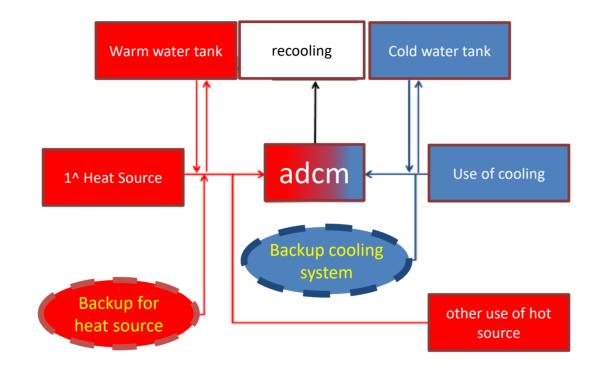
Backup of heat source as CHP, gas boiler, fuel cell... and Backup of cooling system, or a HYBRID CHILLER
